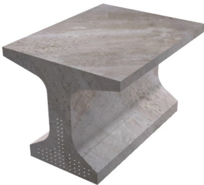
Figure 8- Precast Bulb Tee
