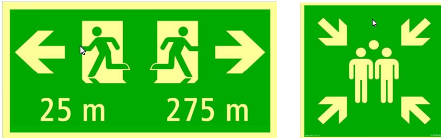
Figure 2.2 - Examples for evacuation signage with distances to the exit emergency exit / cross-passage (left) and the signaling the collection point (right) from [13]
