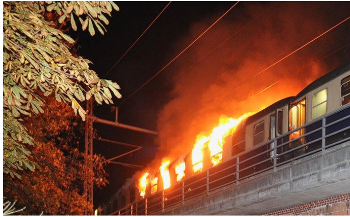
Figure 3.5– Flames and hot smoke gases through several burst windows
